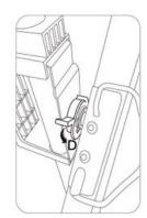
5. With the dial knob on the handle hatch, it is possible to remove the entire housing case of the screen. This is done by turning the dial knob downwards as shown on the picture.
