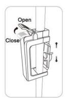
6. After turning the dial knob, the Housing case is then removed as shown.
