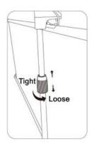
3. Adjust the tightening lock of the Tripod pole, to change the desired height of the of the screen.
