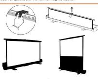
4. When retracting the screen, slowly pull the handle indicated with the yellow label downwards, until the screen has completely retracted back into the casing
