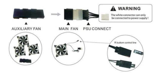
From the main fan (fan in the back) you will in addition to the Molex power cable find a 2-pin cable which plugs into "reset SW" coming from the front of the case. The setup is now complete to control the fans by the front button.
